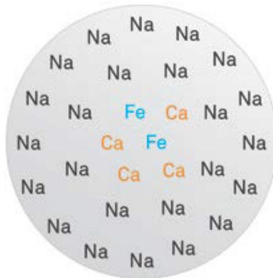
Standard resin beads are susceptible to fouling and leakage as the reaction force decreases as regenerant makes its way through the bead.
