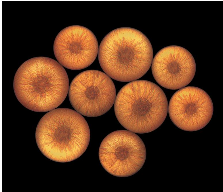
Under a microscope, SST resin looks different because each bead has an inert core that resists fouling and enables more thorough regeneration of the bead.
