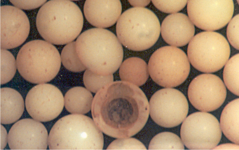
1. Iron oxide fouling of resin center
